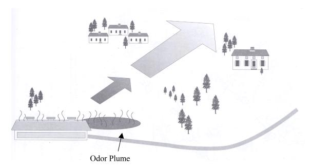
Figure 1. Odor plume and dispersion for a livestock building emitting odor (1).
