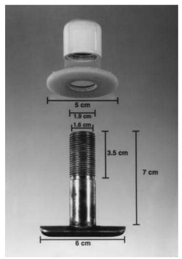
Figure 1. Cannula used in the experiment.
